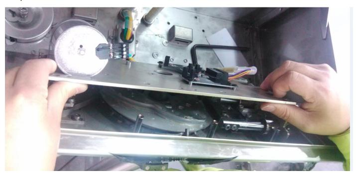
8. There are two electromagnets on the two side of the shaft, please you can select one to hobble it by using the ribbon (according to your requirement, for example if you want the Left-Normal Open, please hobble the electromagnet on the left ).
