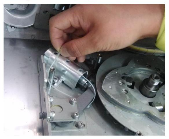
10 Disconnect the power supply of the electromagnet.
