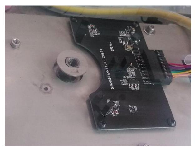
13. Screw up the screw at the gap of the roundel (as the below image shows).
