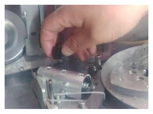
11. Install the mask, please make sure to hold the big electromagnet at the same time, then screw up all the screws around the mask.
