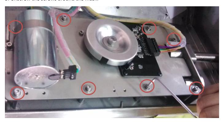
6. Unscrew the screws of the shaft.
